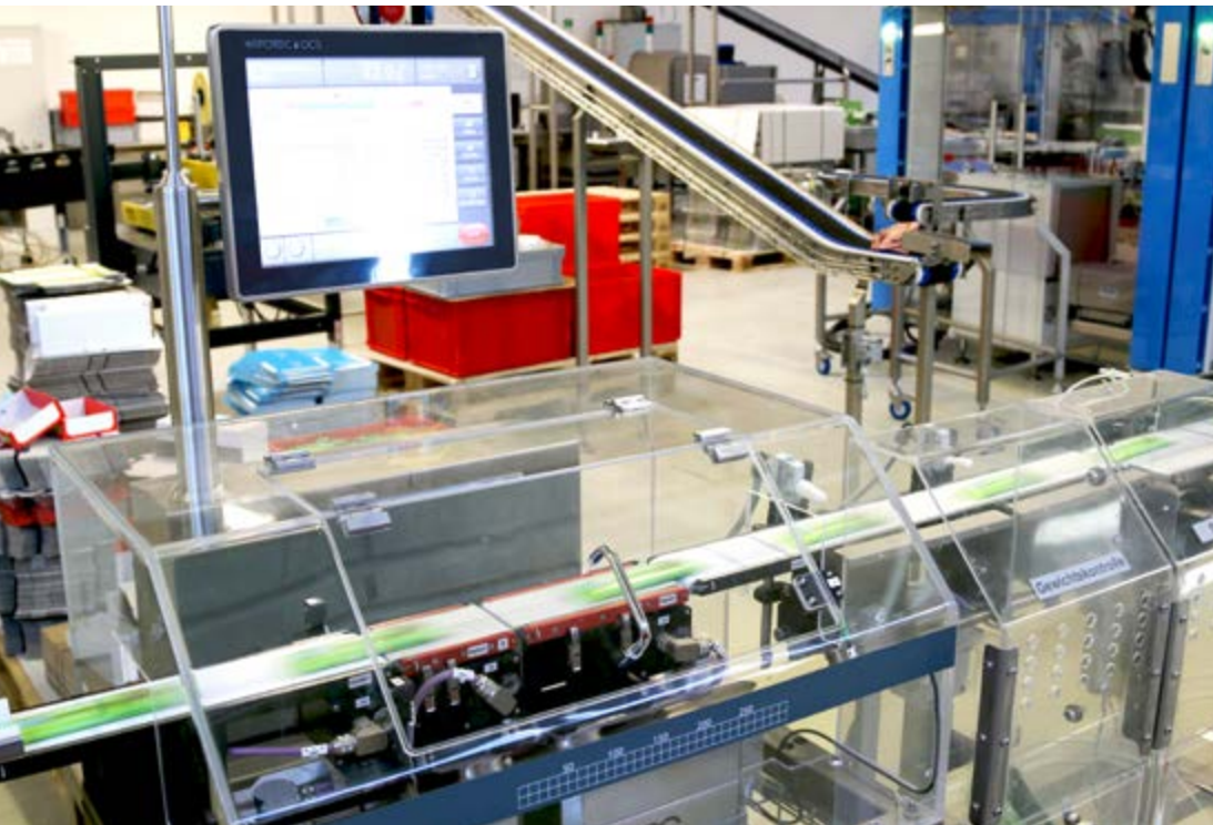
Fruit bars: Over the double scale one after another at maximum speed. Its technology enables minimum product gaps.
