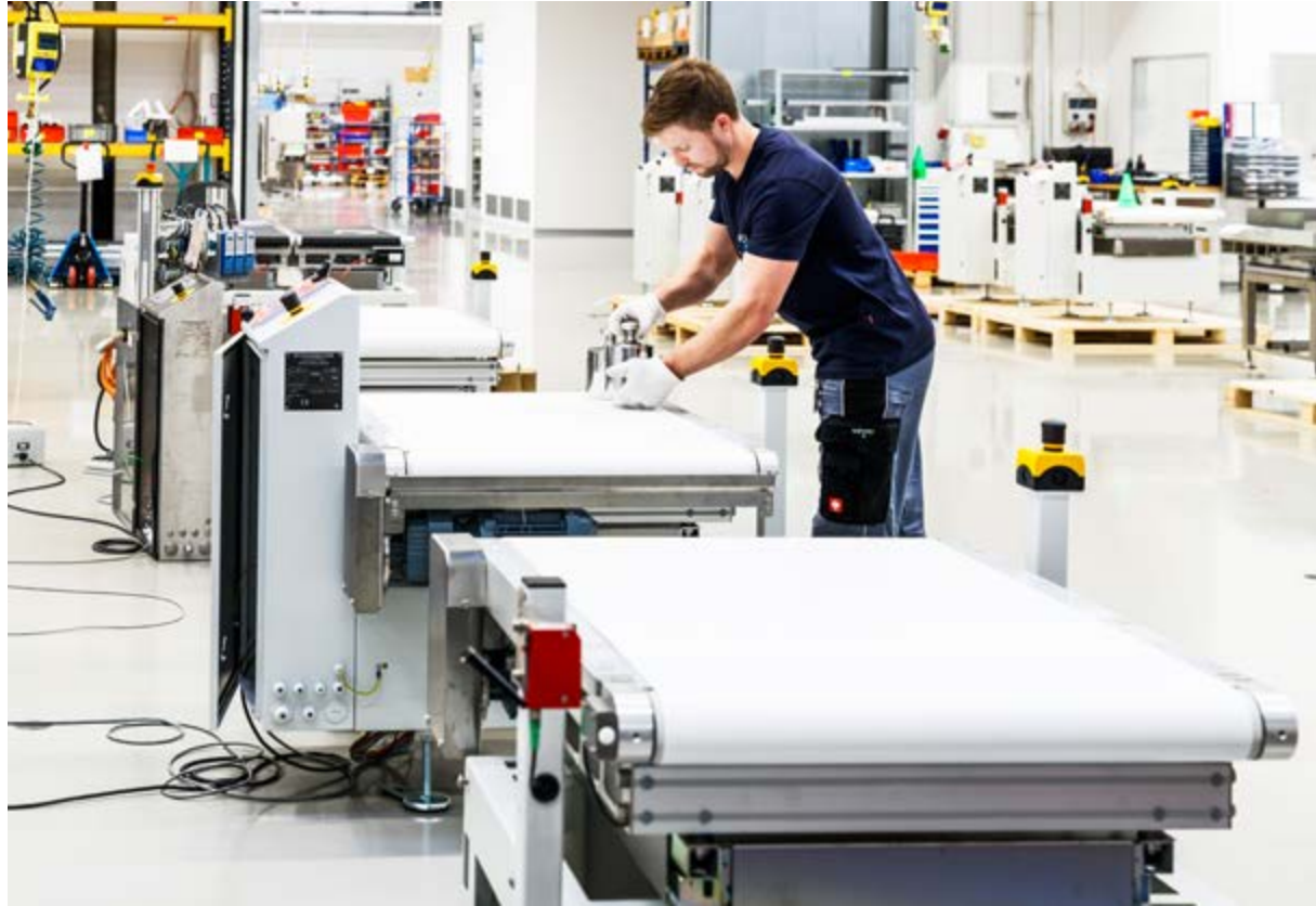
Final acceptance and testing of a heavy load checkweigher
