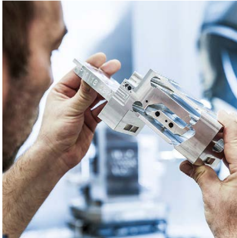
Right: The monoblock, the heart of all WIPOTEC weigh cells
